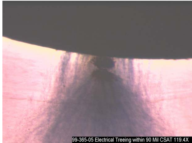
Electrical Tree Initiating through the conductor shield
