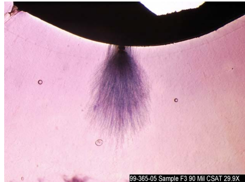
■ #2 AWG XLPE cable from Fullerton. Water treeing more than 40% through the insulation.
