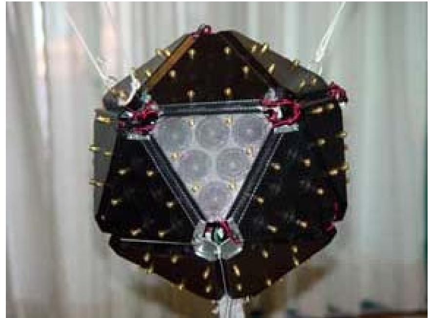
Berkeley Center for New Music and Audio Technology (CNMAT) created a compact loudspeaker array: 10-inch-diameter icosahedron incorporating 120 tweeters.
