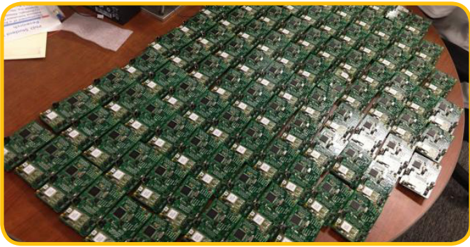
These NeoMotes, data loggers fitted with transceivers, were attached to sensors in each snow-monitoring station. Designed for this project by Professor Steve Glaser and his former student Branko Kerkez, the motes are now commercially manufactured by Metronome Systems in San Jose.
